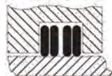
YSD Series QSD Series External - Medium/Heavy Duty 1 set = 2 individual rings (rings rotate with shaft only)
